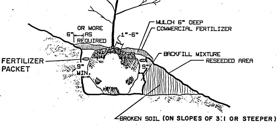
THE TOP OF THE ROOT BALL SHALL BE 2 INCH ABOVE THE NORMAL GROUND LINE IN AVERAGE SOILS, 3 INCHES IN HEAVY CLAY SOILS AND 6 INCHES WHERE IMPERMEABILITY IS ENCOUNTERED.
