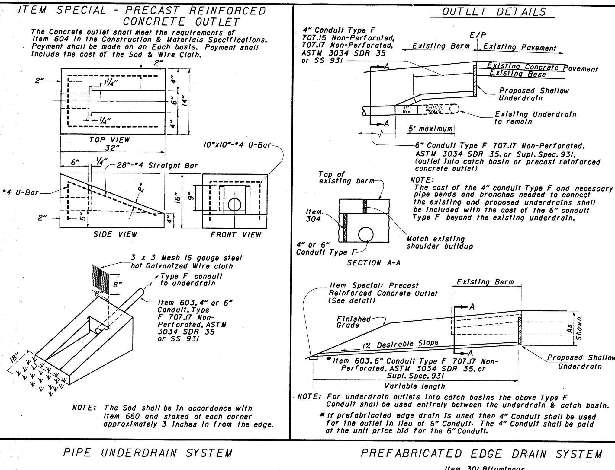
DESCRIPTION: The item shall consist of furnishing and installing a pipe underdrain system or prefabricated edge drain system in accordance with the specifications, details as shown on the plans, and as directed by the Engineer.
