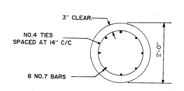
DRILLED SHAFT REINFORCING DETAIL
