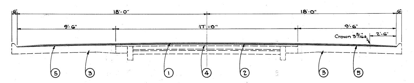
T-35 14 Asphaltic Concrete Surface Course - Type "B" or Type "B" Modified as per special provision.
