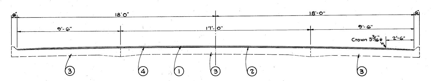
1 T-35 1/4" Asphaltic Concrete Surface Course - Type"B" or Type "B" Modified as per special provision.
