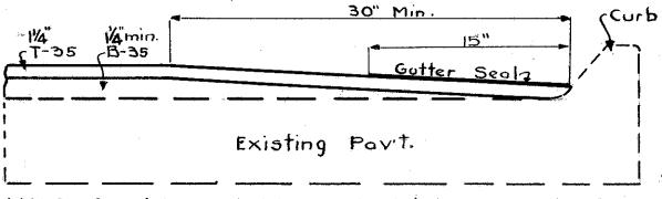
NOTE Special care shall be exercised during construction to obtain maximum comportion of bituminous concrete in all gutters.
