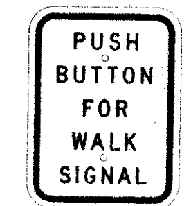
TYPICAL SIGN FOR PED. PUSHBUTTONS
