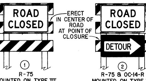
MOUNTED ON TYPE III PORTABLE BARRICADE
