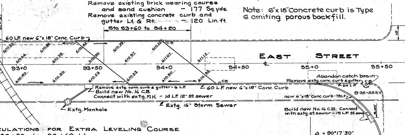
CALCULATIONS FOR EXTRA LEVELING COURSE Sta. 92+90 to 93+60 Lt. (70 x 9 x 1 + 12) + 27 = 1.9 Cu. yds.Sta. 93+60 to 94+20 t. (60 x 29.5 x 3 + 12) + 27 = 16.4 Cu. yds.Sta. 94+30 to 94+50 t. (20 x 9 x 1 + 12) + 27 = 0.6 Cu. yds.Sta. 95+00 to 95+20 Rt. (20 x 9 x 1 + 12) + 27 = 0.6 Cu. yds.(20 x 9 x 1 + 12) + 27 = 0.6 Cu. yds.
