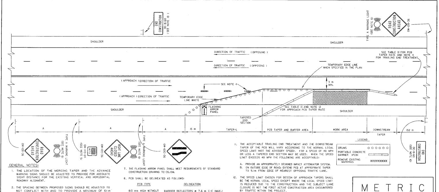
ALL WORK AND TRAFFIC CONTROL DEVICES SHALL BE IN ACCORDANCE WITH 614 AND OTHER APPLICABLE PORTIONS OF THE C & M SPECIFICATIONS AS WELL AS IN ACCORDANCE WITH PART 7 OF THE OMUTCD, PAYMENT FOR ALL LABOR, EQUIPMENT AND MATERIALS TO PROVIDE THIS METHOD OF TRAFFIC CONTROL SHALL BE INCLUDED IN THE LUMP SUM BID FOR 614 MAINTAINING TRAFFIC, UNLESS SEPARATELY ITEMIZED IN THE PLAN.
