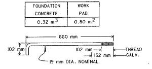
PEDESTAL ANCHOR BOLT ASTM A307 STEEL
