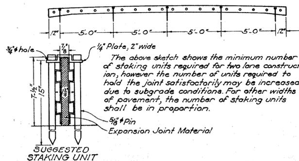
CONTRACTION JOINTS. Contraction joints shown are to be considered as alternates, the type to be used on any project shall be optional with the contractor; and shall be constructed as shown herewith. Contraction joints shall be spaced so that the length of any slab between transverse joints shall not exceed 60 feet. Joint arrangement at intersections shall be as specifically shown on the plans.
