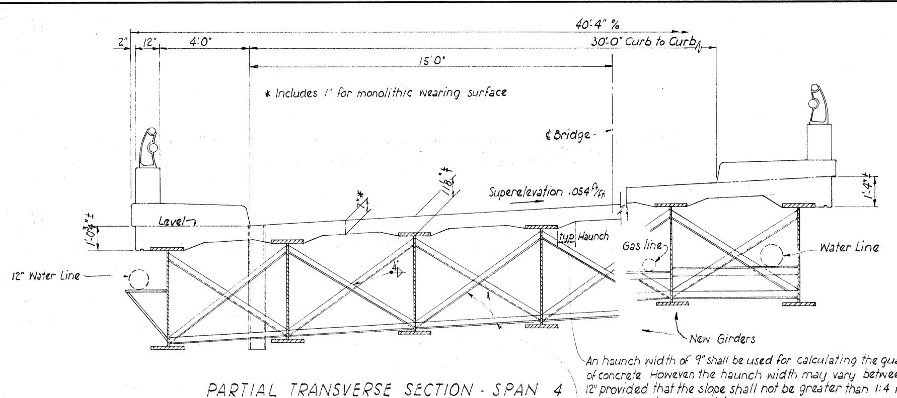
An haunch width of 9" shall be used for calculating the quantity of concrete. However, the haunch width may vary between 6"and 12" provided that the slope shall not be greater than 1:4 for an haunch less than 9" wide.
