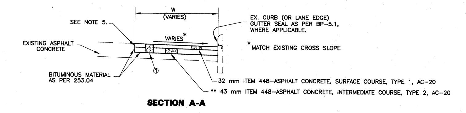
1 TEM 253 - PAVEMENT REPAIR, AS PER PLAN (75 mm MINIMUM DEPTH \*\*)
