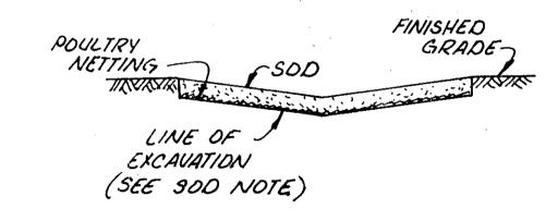
DEPTESSED SHOULDER: THIS PORTION OF THE SHOULDER SHALL BE DEPRESSED TO ASSURE POSITIVE DRAINAGE INTO THE GABION FLUME. ESPECIALLY IN THE SHOULDER AREA IT IS IMPORTANT TO EXCAVATE AND SHAPE THE SUBGRADE ACCORDING TO THE CROSS SECTIONS.
