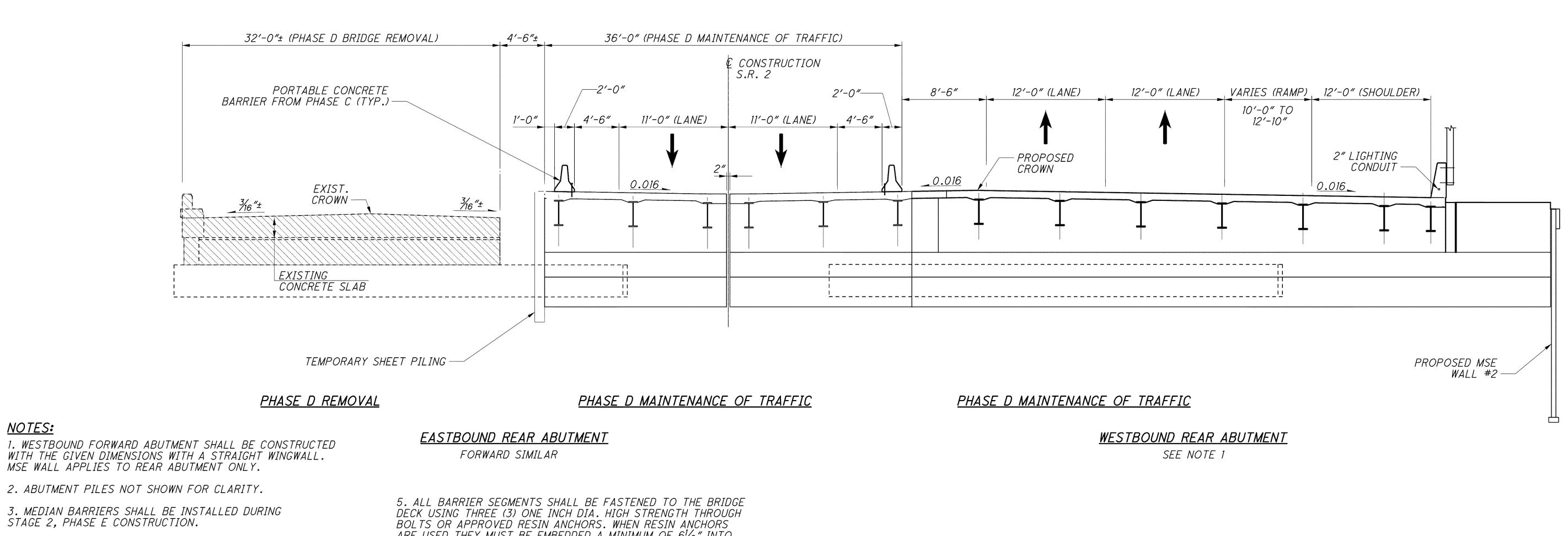
3. MEDIAN BARRIERS SHALL BE INSTALLED DURING STAGE 2, PHASE E CONSTRUCTION. ARE USED THEY MUST BE EMBEDDED A MINIMUM OF 61/2" INTO 4. ALL PHASES SHALL BE CONSTRUCTED IN STAGE 2 AS SHOWN, HOWEVER, LIMITED SUBSTRUCTURE WORK MAY PROCEED DURING SIDE OF THE BARRIER WITH THE ANCHOR PATTERN SYMMETRICAL STAGE 1 (PHASE B), AS APPROVED BY THE ENGINEER. ABOUT THE CENTER OF EACH SEGMENT.
