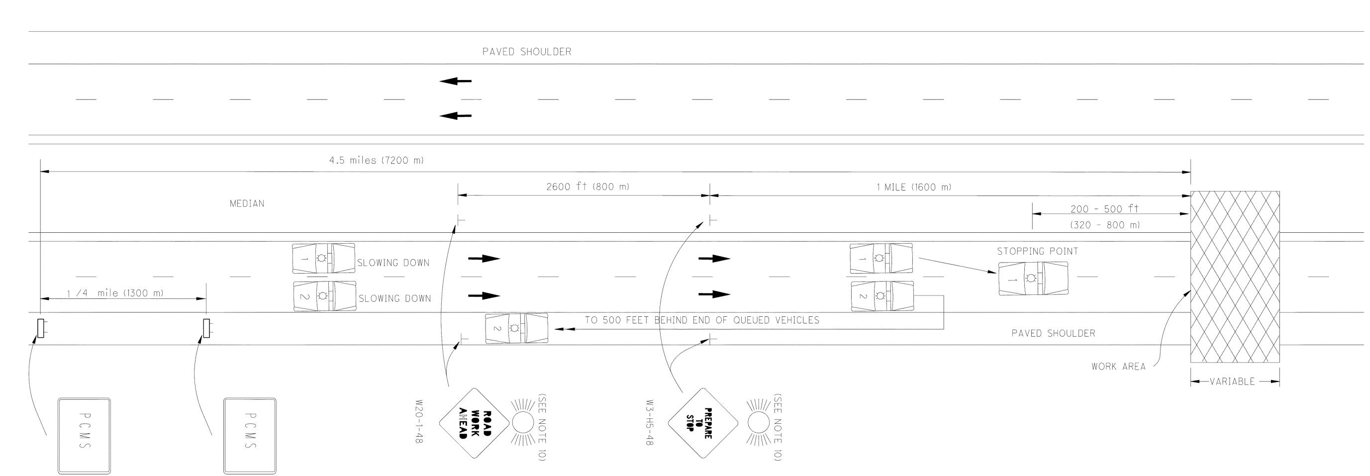
This type of highway closure shall be used for all construction, maintenance and utility operations when the duration of closure will not exceed 15 minutes.
