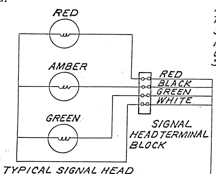
CABLE SHALL BE RUN INTO SIGNAL HEAD AND CONNECTIONS ARE TO BE MADE AT TERMINAL BLOCK. WHEN TWO 4-CONDUCTOR CABLES ARE USED AT FIRST HEAD FROM CONTROLLER BOTH CABLES SHALL BE CONNECTED AT TERMINAL BLOCK IN HEAD.
