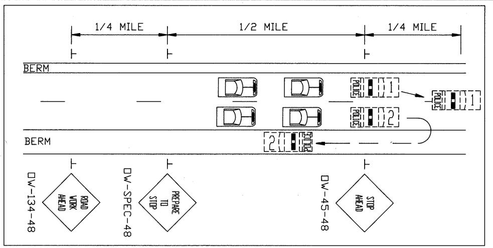
NOTE: DETAIL IS SHOWN FOR TWO LANE DIRECTIONAL TRAFFIC. IF ADDITIONAL DIRECTIONAL LANES EXIST, THE STOPPAGE OF TRAFFIC SHALL BE ACCOMPLISHED IN ACCORDANCE WITH THE EXISTING ROADWAY CONDITIONS.
