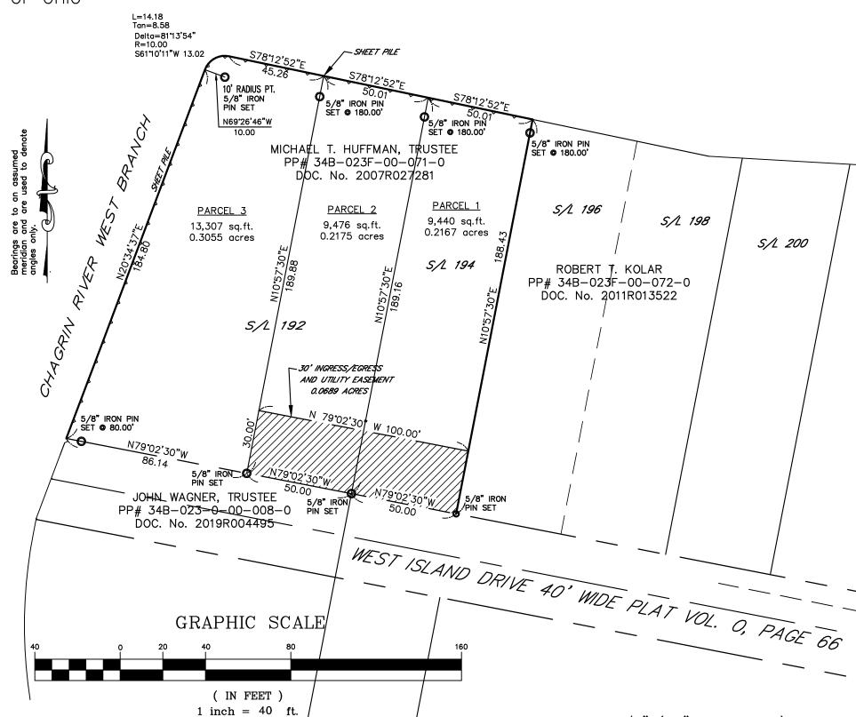
ALL IRON PINS SET ARE 5/8" (30" OF LENGTH) AND ARE IDENTIFIED BY A PLASTIC CAP BEARING
