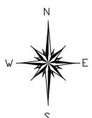
BASIS OF BEARINGS ARE TO AN ASSUMED MERIDIAN ALONG THE CENTERLINE OF SOM CENTER ROAD NORTH 01°-11'-52" WEST
