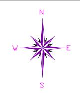
BASIS OF BEARINGS ARE TO AN ASSUMED MERIDIAN ALONG THE NORTH 89°-48'-26" FAST STATE PLANE COORDINATES, NAD 83 2011, OHIO NORTH ZONE, GEOID 12 B
