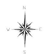
BASIS OF BEARINGS ARE TO AN ASSUMED MERIDIAN ALONG THE CENTERLINE OF NORTH STATE STREET NORTH 44°-23'-06" WEST
