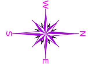
BASIS OF BEARINGS ARE TO AN ASSUMED MERIDIAN ALONG THE CENTERLINE OF AUBURN ROAD NORTH  $06^{\circ}-08'-58''$  WEST
