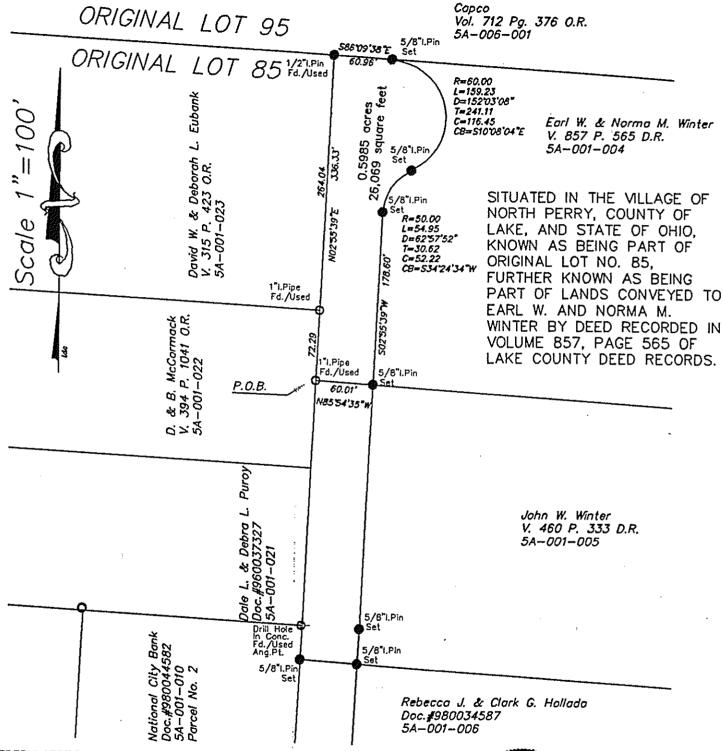
I HEREBY CERTIFY THAT THIS PLAT WAS PREPARED FROM A FIELD SURVEY MADE UNDER MY DIRECT SUPERVISION. MONUMENTS WERE FOUND OR SET AS INDICATED. DIMENSIONS ARE EXPRESSED IN FEET AND DECIMAL PARTS THEREOF. BASIS OF BEARINGS IS THE CENTERLINE OF ANTIOCH ROAD, NORTH 00'30'00" EAST. ALL OF WHICH ARE CORRECT TO THE BEST OF MY KNOWLEDGE AND BELIEF. THIS PLAT WAS PREPARED IN ACCORDANCE WITH THE PROVISIONS OF CHAPTER 4733—37 IF THE OHIO ADMINISTRATIVE CODE.
