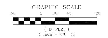
DISTANCES ARE SHOWN IN FEET AND DECIMAL PARTS THEREOF. BEARINGS SHOWN ARE BASED ON AN ASSUMED MERIDIAN AND ARE USED TO DESCRIBE ANGLES ONLY.
