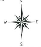
BASIS OF BEARINGS ARE TO AN ASSUMED MERIDIAN ALONG THE CENTERLINE OF NORTH RIDGE ROAD NORTH 82°-27'-50" WEST
