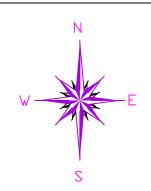
BASIS OF BEARINGS ARE TO AN ASSUMED MERIDIAN ALONG THE CENTERLINE OF BATES ROAD NORTH 01°-00'-52" WEST STATE PLANE COORDINATES, NAD 83 2011, OHIO NORTH ZONE, GEOID 12 B
