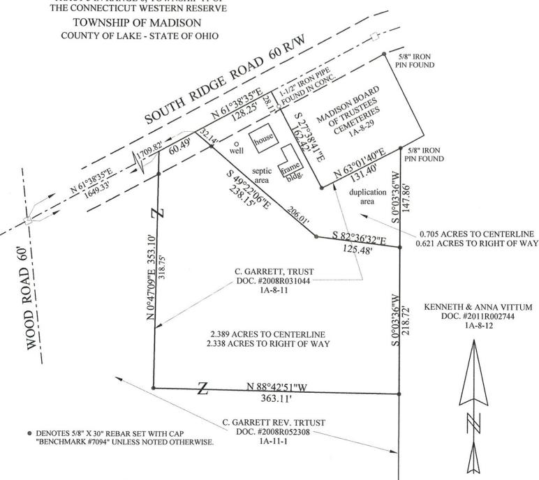
THIS MAP OF SURVEY REPRESENTS A TRUE FIELD SURVEY PERFORMED BY ME ON FEBRUARY 27, 2016. BEARINGS SHOWN HEREON ARE TO AN ASSUMED MERIDIAN AND ARE USED TO DENOTE ANGLES ONLY. IRON PINS SET ARE 5/8" X 30" REBAR CAPPED "BENCHMARK #7094". DISTANCES ARE EXPRESSED IN FEET AND DECIMAL PARTS THEREOF IN ACCORDANCE WITH OHIO ADMINISTRATIVE CODE 4733-37.
