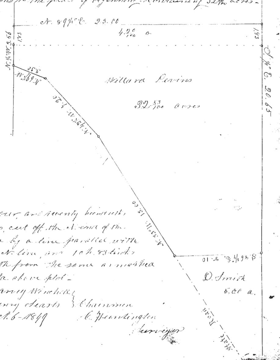
Four and seventy hundredths acres, cut off the N. end of the above by a line parallel with the N. line, and 1 ch. 83 links south from the same as marked on the above plot -
