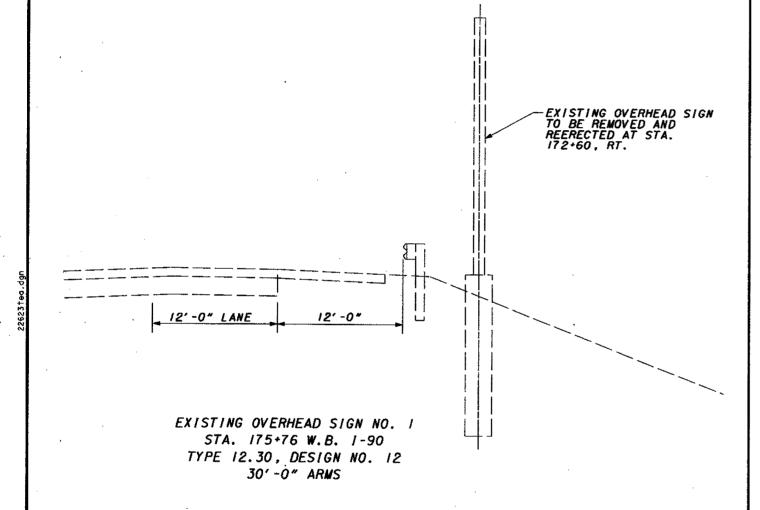
8'-0"x2'-0"<del>- 9'-0"</del> <u>GEP-84</u> EXIT 189 91 Willoughby Hills Willoughby 1/2MILE 29'-0" POLE (FROM STA. 175+76, RT.) 21' -0"x 12' -0" GB-11 12'-0" RIGID OVERHEAD -SIGN SUPPORT FOUNDATION PROPOSED OVERHEAD SIGN NO. 2 -685± STA. 172+60 W.B. 1-90 TYPE 12.30, DESIGN NO. 12 30'-0" ARMS
