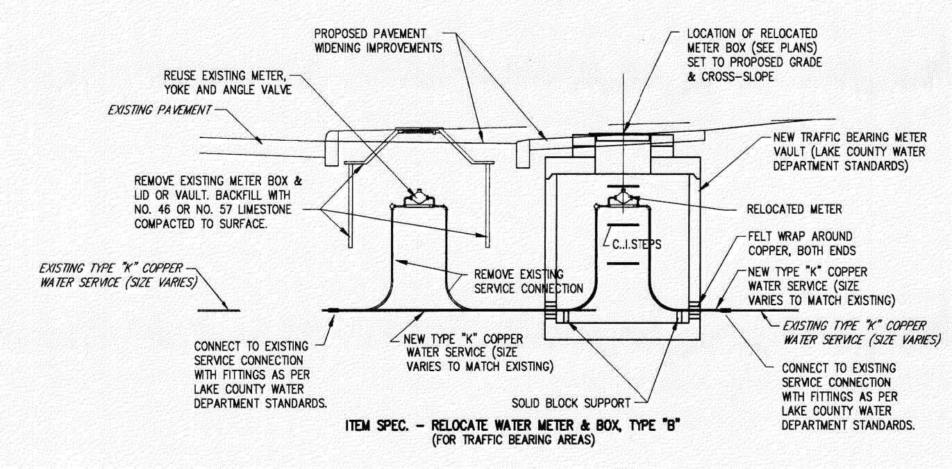
THIS ITEM SHALL INCLUDE FURNISHING ALL LABOR, MATERIALS AND EQUIPMENT NECESSARY TO RELOCATE THE EXISTING WATER METER AND PROVIDE A NEW WATER METER VAULT IN ACCORDANCE WITH THE LAKE COUNTY WATER DEPARTMENT STANDARDS, INCLUDING EXCAVATION, DEWATERING, SHEETING, BACKFILL AND ALL OTHER INCIDENTAL MATERIALS AND/OR EXPENSES REQUIRED, WHETHER SPECIFICALLY MENTIONED OR NOT.
