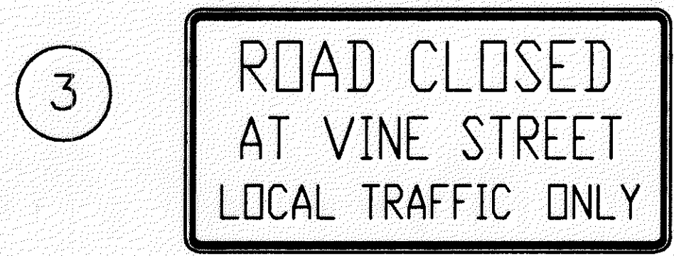
3 R-76A 1524mmX762mm(60"X30") & OC-14L 1219mmX610mm(48"X24") WITH TYPE III BARRICADE
