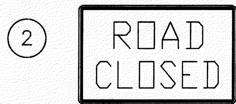
2 R-75 1219mmX762mm(48"X30") & OC-14R 1219mmX610mm(48"X24") WITH TYPE III BARRICADE
