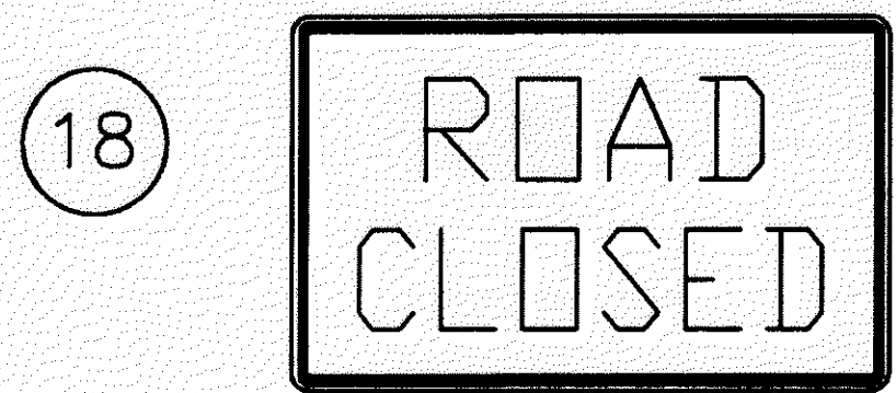
18 R-75 1219mmX762mm(48"X30") & OC-14L 1219mmX610mm(48"X24") WITH TYPE III BARRICADE
