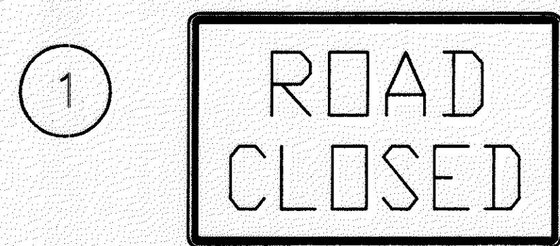
1 R-75 1219mmX762mm(48"X30") WITH TYPE III BARRICADE
