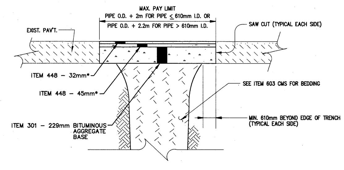
1) EXISTING SUBBASE MATERIAL (IF ANY) SHALL BE REPLACED, AS DIRECTED BY ENGINEER.
