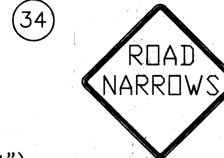
34 OW-51-36 (61 METERS PRIOR TO WORK ZONE)
