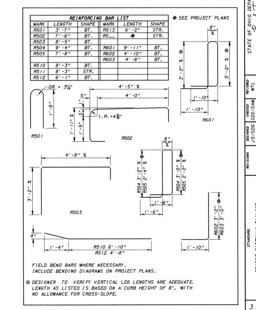
DGE SIDEWALK RAILING TH CONCRETE PARAPETS
