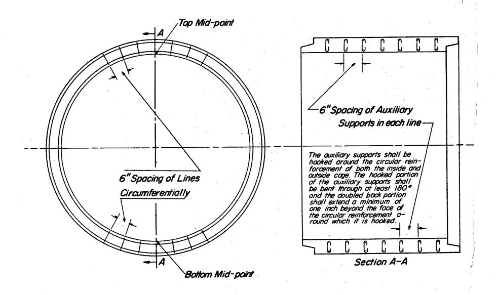
Sketch of Auxiliary Support System For 60" Diameter Pipe (No. 2 @ 6";7 lines @ 6")
