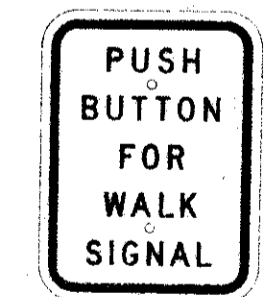
TYPICAL SIGN FOR PED. PUSHBUTTONS
