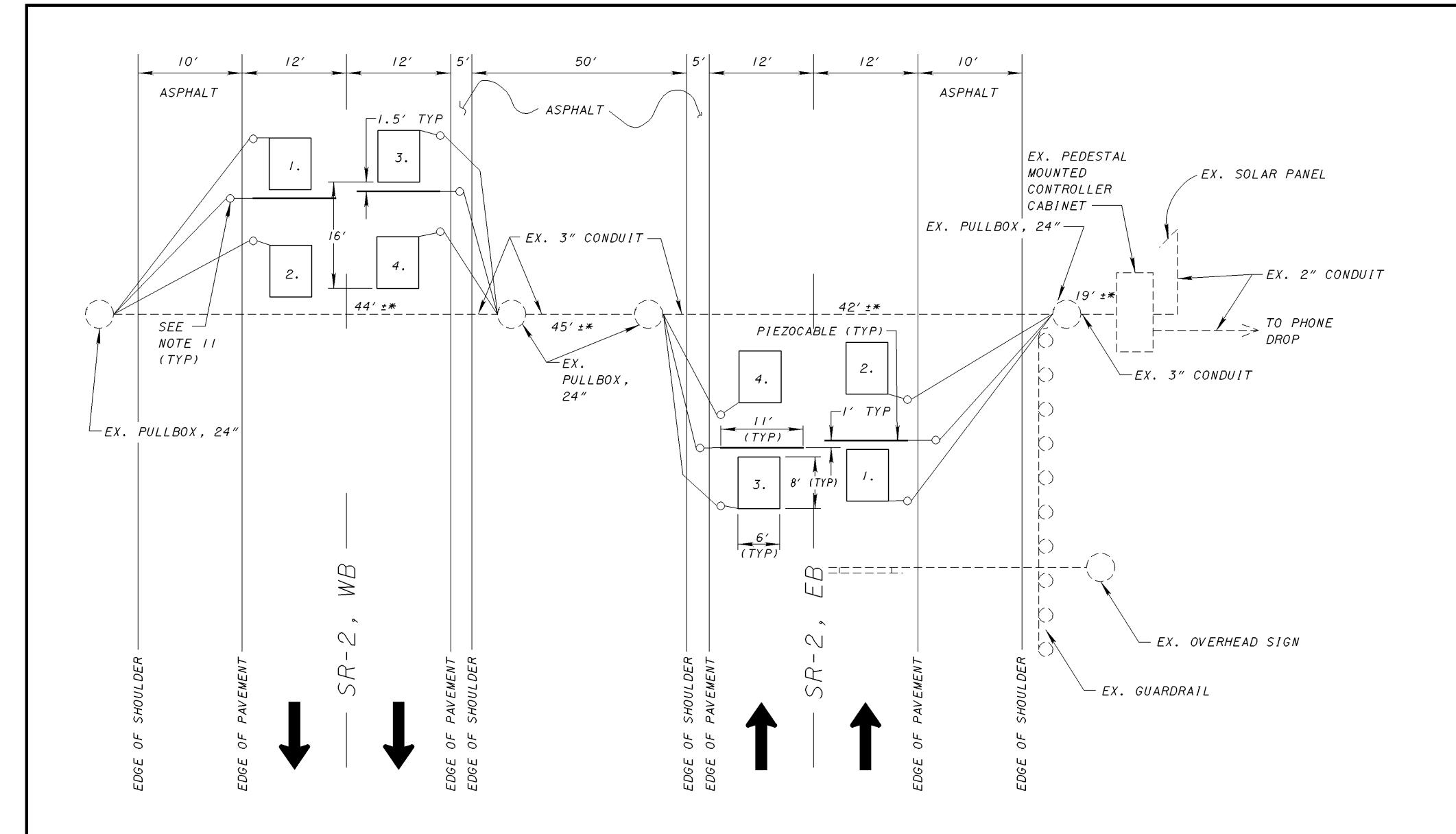
LAK-2: WEST OF SR-615 STA 380+25 ± CONTROLLER IN EB DIRECTION, BEHIND EXISTING GUARDRAIL
