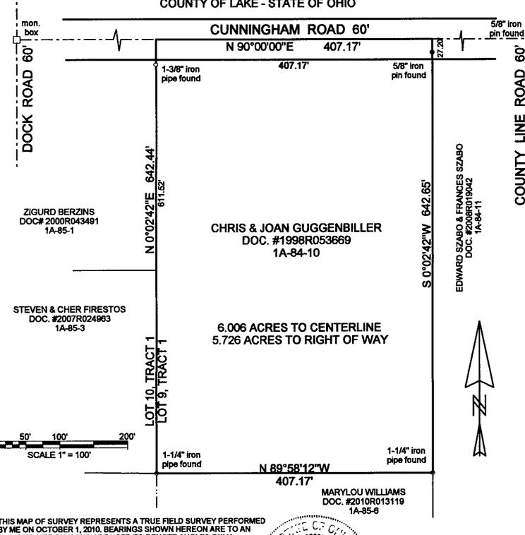
THIS MAP OF SURVEY REPRESENTS A TRUE FIELD SURVEY PERFORMED BY ME ON OCTOBER 1, 2010. BEARINGS SHOWN HEREON ARE TO AN ASSUMED MERIDIAN AND ARE USED TO DENOTE ANGLES ONLY.
