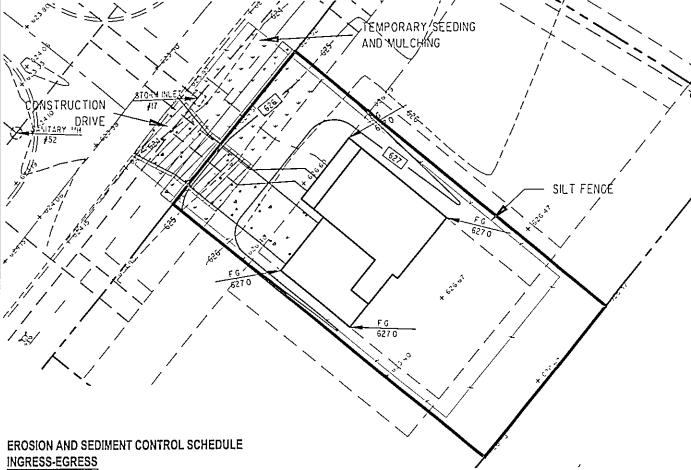
A STONE ACCESS DRIVE COMPLETE WITH UNDER LYING GEO-TEXTILE FABRIC (20 FEET WIDE AND 50 FEET LONG) FOR INGRESS AND EGRESS AT THE SITE SHALL BE INSTALLED. THIS DRIVE SHALL BE THE ONLY ENTRANCE AND EXIT TO THE SITE.
