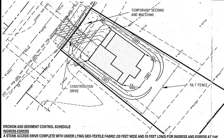
A STONE ACCESS DRIVE COMPLETE WITH UNDER LYING GEO-TEXTILE FABRIC (20 FEET WIDE AND 50 FEET LONG) FOR INGRESS AND EGRESS AT THE SITE SHALL BE INSTALLED. THIS DRIVE SHALL BE THE ONLY ENTRANCE AND EXIT TO THE SITE.
