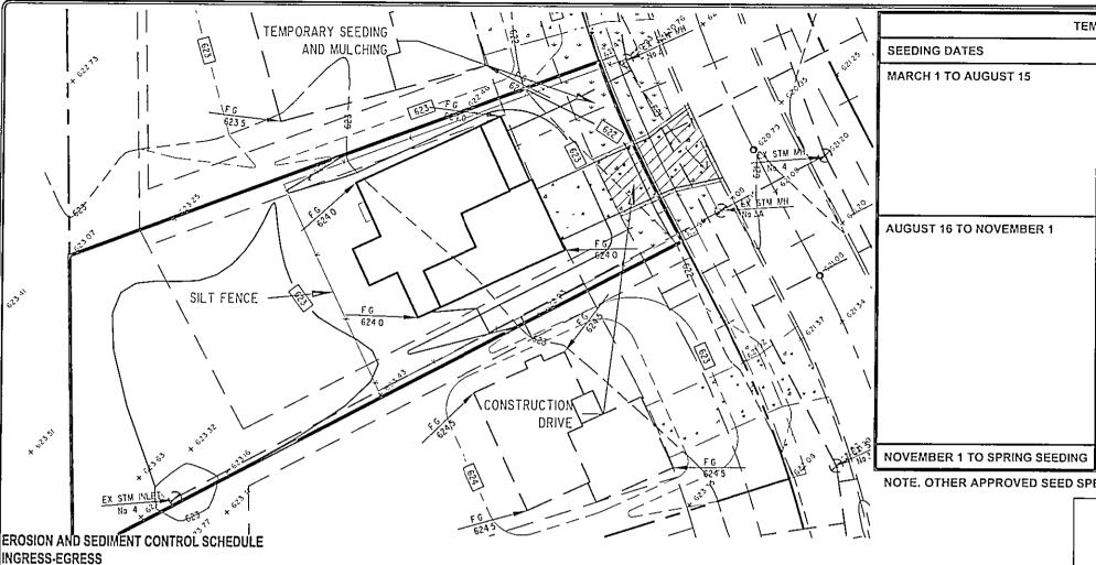
A STONE ACCESS DRIVE COMPLETE WITH UNDER LYING GEO-TEXTILE FABRIC (20 FEET WIDE AND 50 FEET LONG) FOR INGRESS AND EGRESS AT THE SITE SHALL BE INSTALLED. THIS DRIVE SHALL BE THE ONLY ENTRANCE AND EXIT TO THE SITE.
