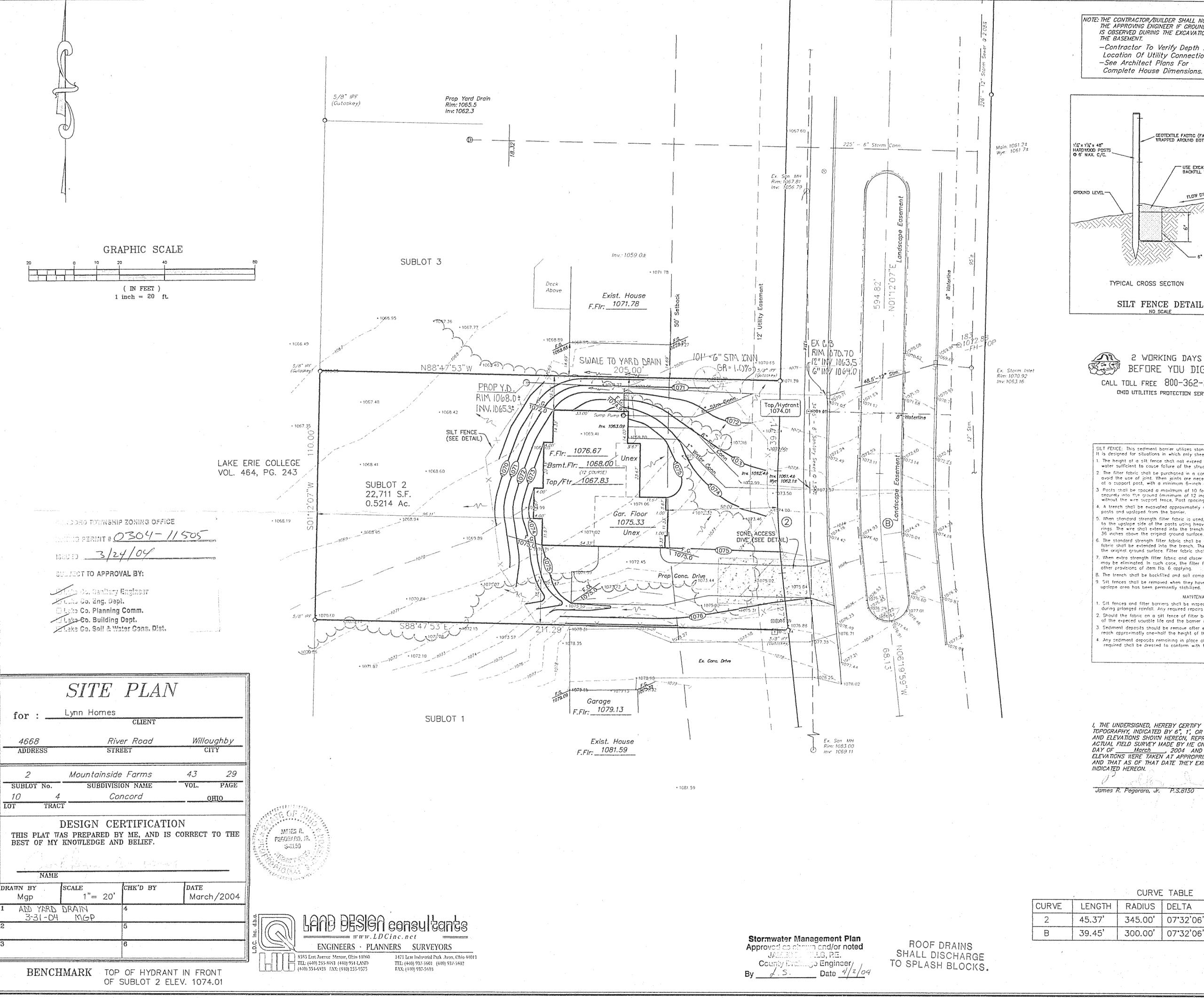
NOTE: THE CONTRACTOR/BUILDER SHALL NOTIFY THE APPROVING ENGINEER IF GROUNDWATER IS OBSERVED DURING THE EXCAVATION OF THE BASEMENT.
