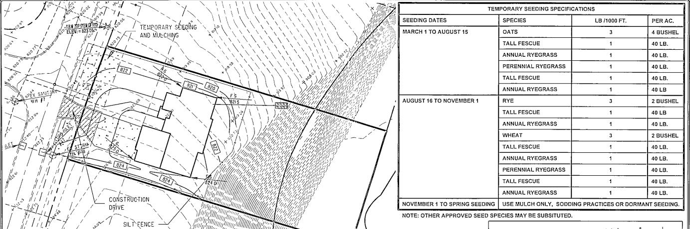
ingress-egress A STONE ACCESS DRIVE COMPLETE WITH UNDER LYING GEO-TEXTILE FABRIC (20 FEET WIDE AND 50 FEET LONG) FOR INGRESS AND EGRESS AT THE SITE SHALL BE INSTALLED. THIS DRIVE SHALL BE THE ONLY ENTRANCE AND EXIT TO THE SITE.
