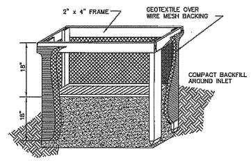
INLET PROTECTION IN SWALES, DITCH LINES OR YARD INLETS
