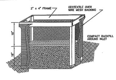
INLET PROTECTION IN SWALES, DITCH LINES OR YARD INLETS
